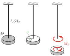
$$\vartheta = \frac{M_T l}{GI_T} \quad c_T = \frac{M_T}{\vartheta} = \frac{GI_T}{l}$$
