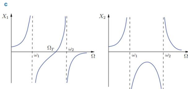
$$m_1 \ddot{x}_1 = -2 \cdot \frac{1}{2} c_1 x_1 + c_2(x_2 - x_1) + F_0 \cos \Omega t,$$
