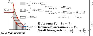
$$p_{2}T_{2}^{\kappa/(\kappa-1)} = p_{1}T_{1}^{\kappa/(\kappa-1)} \Leftrightarrow \frac{p_{2}}{p_{1}} = \left(\frac{T_{1}}{T_{2}}\right)^{\frac{\kappa}{(\kappa-1)}} \qquad \eta = \frac{\text{Nutzen}}{\text{Aufwand}} \qquad \eta_{Otto} = \frac{\mid W_{mech,\odot}^{rev} \mid}{W_{th,\oplus}} = \frac{(T_{3} - T_{2}) + (T_{1} - T_{4})}{(T_{3} - T_{2})} \qquad \text{Entropiestrom}$$
