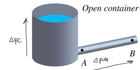
$$\begin{aligned} \Delta p_C - \Delta p_{AB} &= 0 \\ \Delta p_{AB} &= \Delta p_L + \Delta p_R \end{aligned}$$
