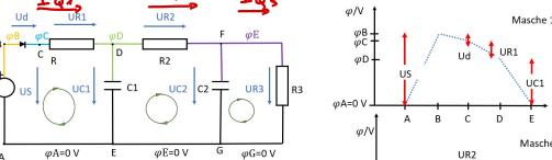
$$\begin{aligned} -U_s + U_d + U_{R1} + U_{C1} &= 0 \\ -U_{C1} + U_{R2} + U_{C2} &= 0 \\ -U_{C2} + U_{R3} &= 0 \end{aligned}$$
