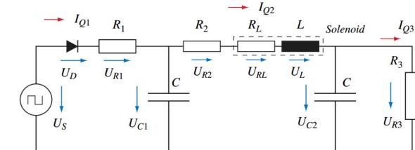
$$\begin{aligned} U_s + U_D + U_{R1} + U_{C1} &= 0 \\ -U_{C1} + U_{R2} + U_{spule} + U_{C2} &= 0 \\ U_{RL} + U_L &= U_{spule} \\ -U_{C2} + U_{R3} &= 0 \end{aligned}$$
